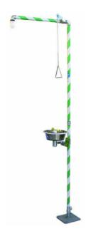
Size Emergency and eye shower MB150-30 (11/4") Article number 99999979 Material Stainless steel bath, Steel pipes, Plastic shower head **Pipework** Galvanized Stainless steel push bar and Operation stainless steel pull bar Water flow Shower 80 ltr/min, bath 12 ltr/min. 11/4" BSP internal thread Water supply
